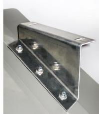
REES – Holder for steps and walking gratings to mount on trapezoidal roofings. Assemble clamp holder on the raised bead with the self-drilling screws. Suitable for roof pitches of maximum 30 degrees. The clamp holder will be manufactured after the client's requests
